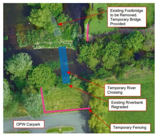
The existing vehicular access to the OPW carpark will be maintained for the duration of the works. A temporary river crossing will need to be constructed for the construction period in order to access the island from the southern side of the river.
